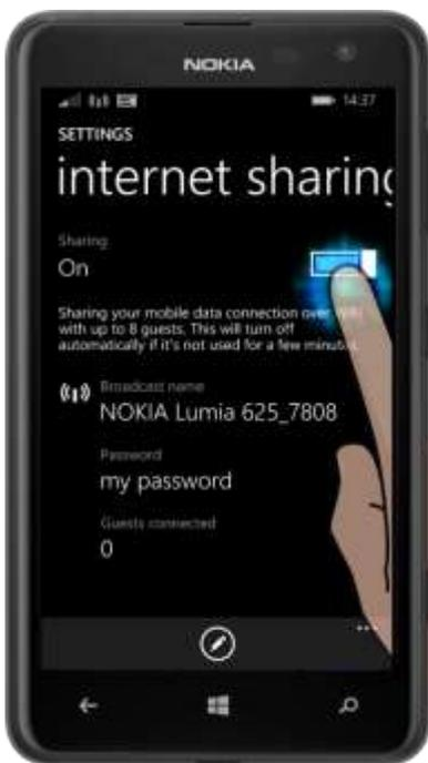
Tap the sharing slider to switch sharing on. You can change the name and password for connecting by tapping the pencil icon at the bottom of the screen.
